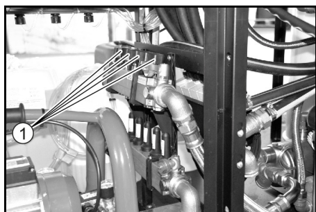
① Washing station heater stop valve
